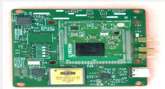
Credit Card size Receiver Module (57mm x 68mm)
