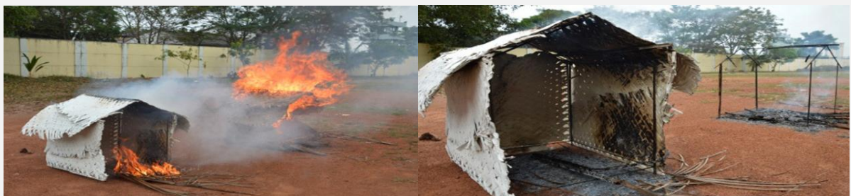
Fig. 1 Model huts made of thatched coconut leaves set to fire. (Left)-Hut without CASPOL coating gutted completely in fire within a few seconds whereas CASPOL coated hut remained intact even in fire.
