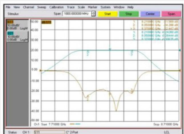
Measured Response of X Band Filter
