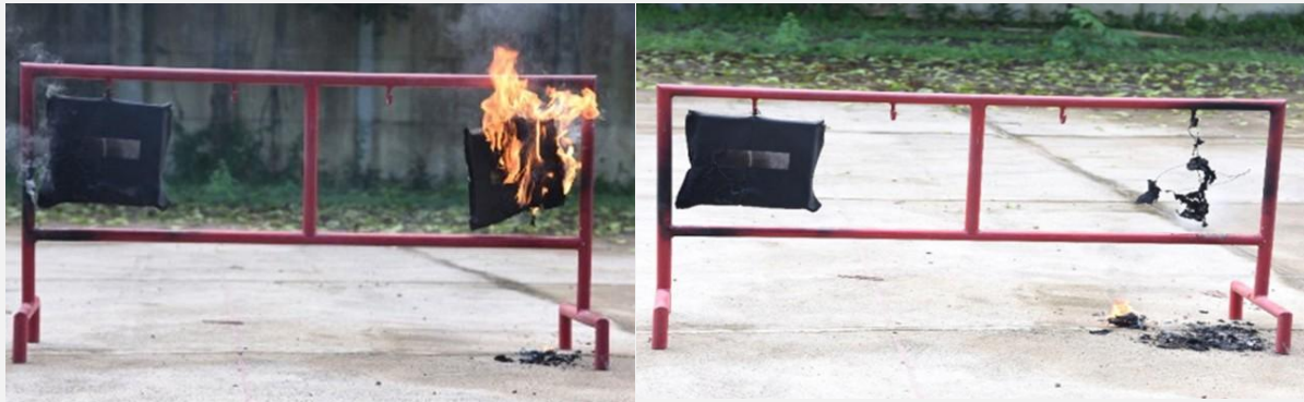
Fig. 3 Two images of commercial seat cushion set to fire. In each image: (Left)-cushion with CASPOL impregnation remain intact even after fire whereas cushion without CASPOL impregnation (Right) is burned completely in fire within a few seconds
