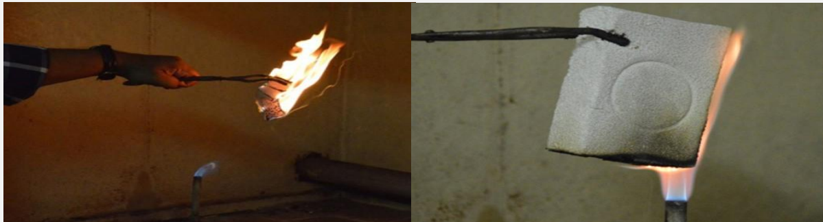
Fig. 2 Images of commercial polyurethane foams set to fire. (Left)-foam without CASPOL impregnation burned completely in fire within a few seconds whereas CASPOL impregnated foam (right) remained intact even in fire.
