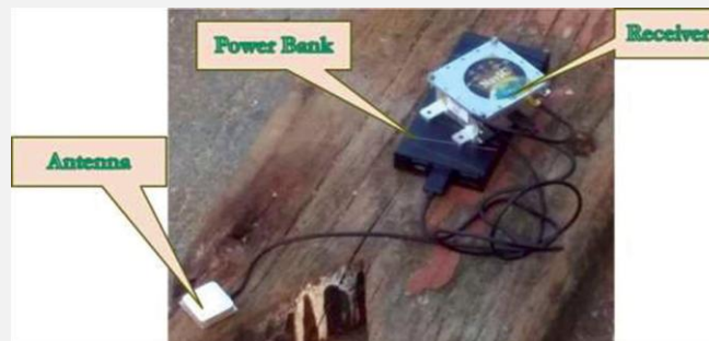
NavIC Messaging and Positioning Receiver Setup with power bank and Antenna
